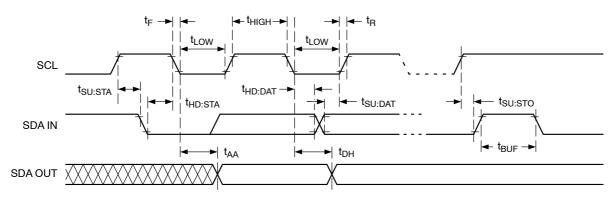
Figure 3. I<sup>2</sup>C Serial Interface Timing
