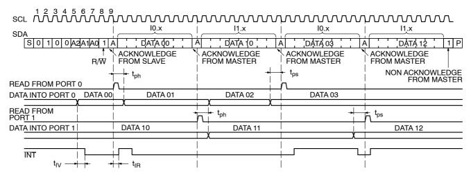
NOTE: Transfer of data can be stopped at any moment by a STOP condition. When this occurs, data present at the latest acknowledge phase is valid (output mode). It is assumed that the command byte has previously been set to 00 (read input port register).
