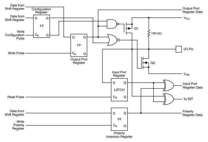
Figure 6. Simplified Schematic of I/Os
