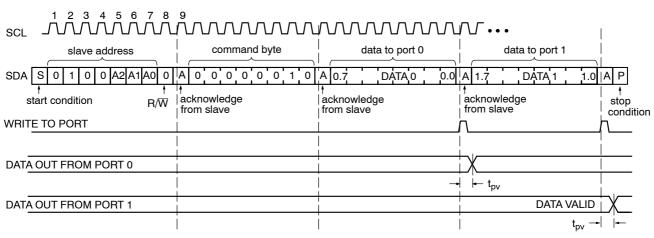
Figure 10. Write to Output Port Register
