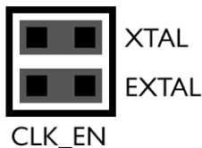
Figure 6-23: External Crystal Circuitry Enable (J22)
