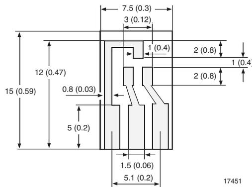
**PACKAGE DIMENSIONS** in millimeters (inches): **SOT-23**
