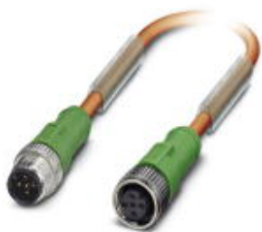
Sensor/actuator cable, 5-position, PUR halogen-free, irradiated, orange RAL 2003, Plug straight M12, A-coded, on Socket straight M12, A-coded, cable length: 1.5 m, Customer version
