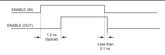
Figure 2-109 • Timing Diagram (option 2: enables skew circuit)
