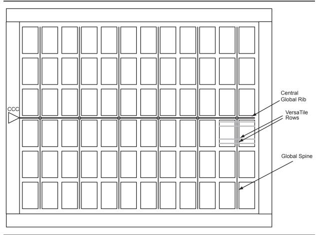
Figure 2-15 • Example of Global Tree Use in an AFS600 Device for Clock Routing
