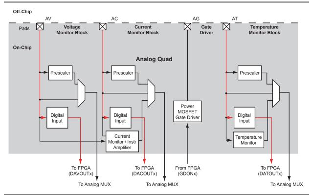
Figure 2-69 • Analog Quad Direct Digital Input Configuration
