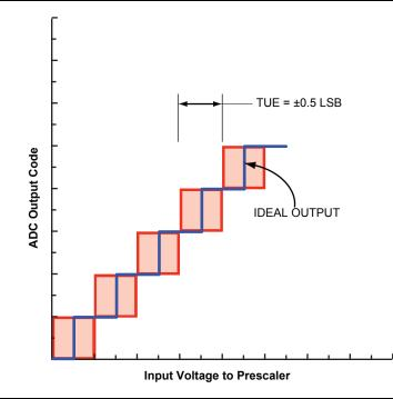
Figure 2-87 • Total Unadjusted Error (TUE)
