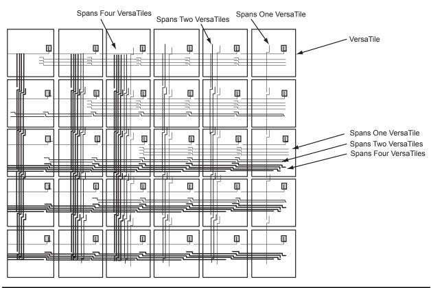
Figure 2-9 • Efficient Long-Line Resources
