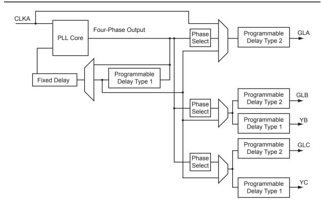
Note: Clock divider and multiplier blocks are not shown in this figure or in SmartGen. They are automatically configured based on the user's required frequencies.
