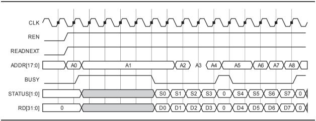
Figure 2-41 • Read Next WaveForm (Pipe Mode, 32-bit access)
