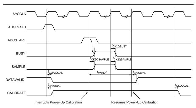
*Note:* \*t<sub>CONV</sub> represents the conversion time of the second conversion. See EQ 23 on page 2-109 for calculation of the conversion time, t<sub>CONV</sub>.
