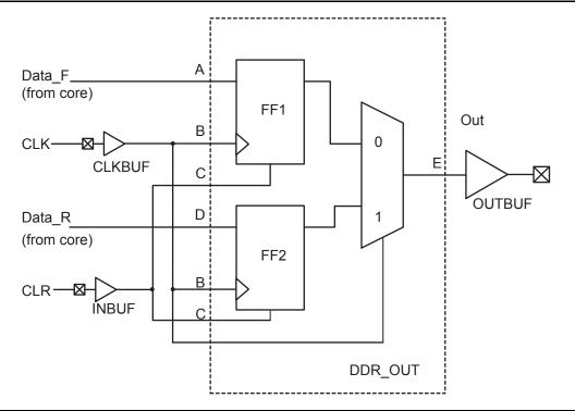
Figure 2-102 • DDR Output Support in Fusion Devices
