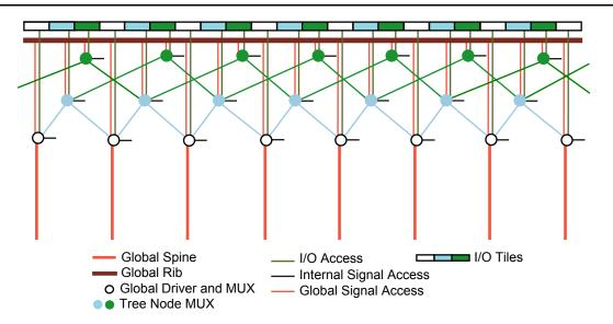
Figure 2-14 • Clock Aggregation Tree Architecture
