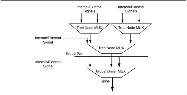
Figure 2-13 • Spine-Selection MUX of Global Tree
