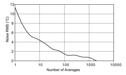
Figure 2-96 • Temperature Reading Noise When Averaging is Used
