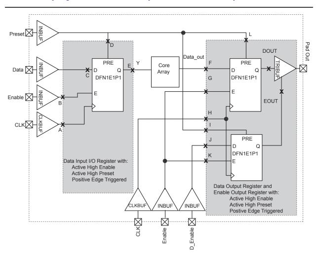
Figure 2-137 • Timing Model of Registered I/O Buffers with Synchronous Enable and Asynchronous Preset
