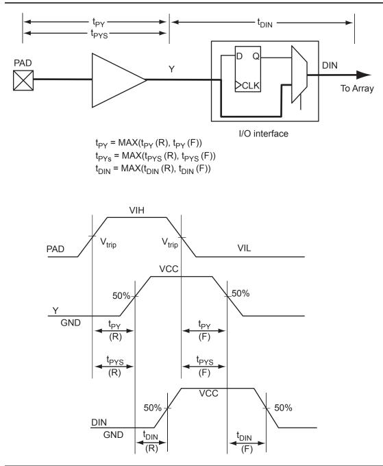
Figure 2-116 • Input Buffer Timing Model and Delays (example)
