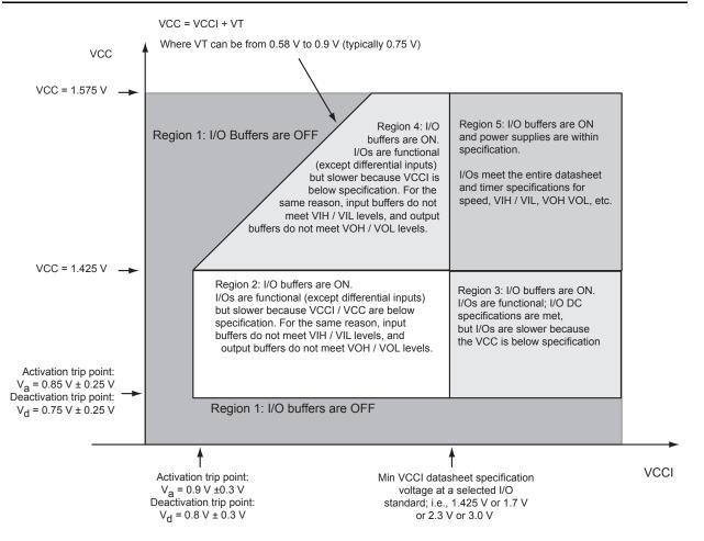
Figure 3-1 • I/O State as a Function of VCCI and VCC Voltage Levels
