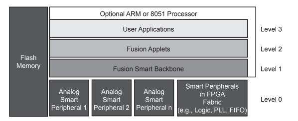
Note: Levels 1, 2, and 3 are implemented in FPGA logic gates.
