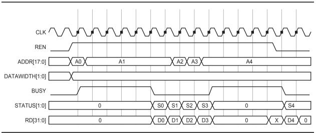
Figure 2-39 • Read Waveform (Pipe Mode, 32-bit access)
