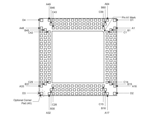
Note: The die attach paddle center of the package is tied to ground (GND).
