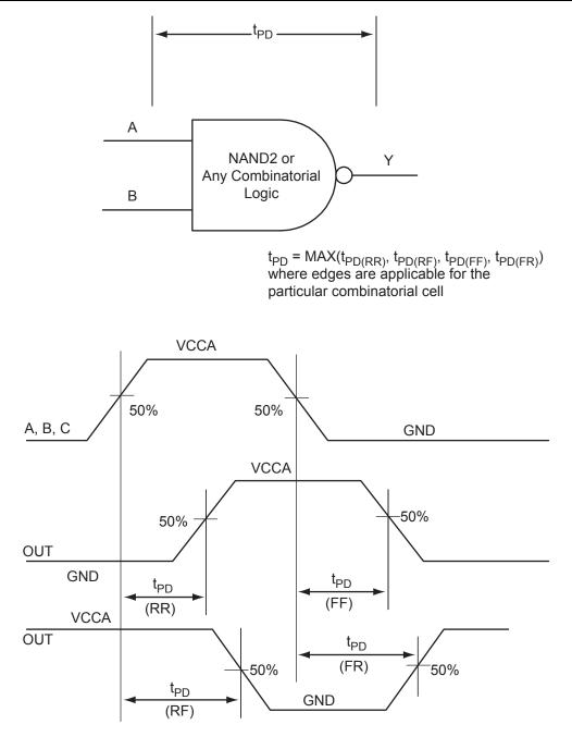
Figure 2-4 • Combinatorial Timing Model and Waveforms
