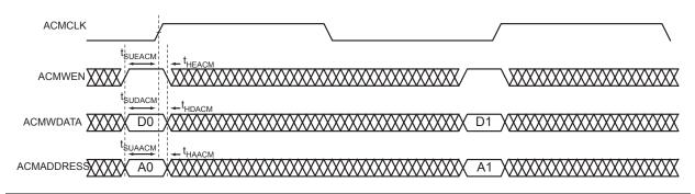
Figure 2-97 • ACM Write Waveform
