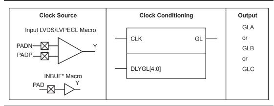
Figure 2-21 • Fusion CCC Options: Global Buffers with Programmable Delay
