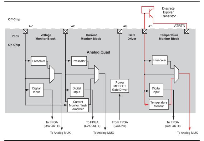
Figure 2-76 • Temperature Monitor Quad
