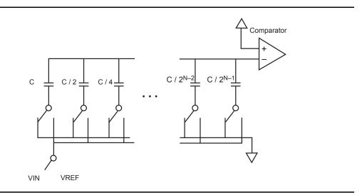
Figure 2-81 • Example SAR ADC Architecture
