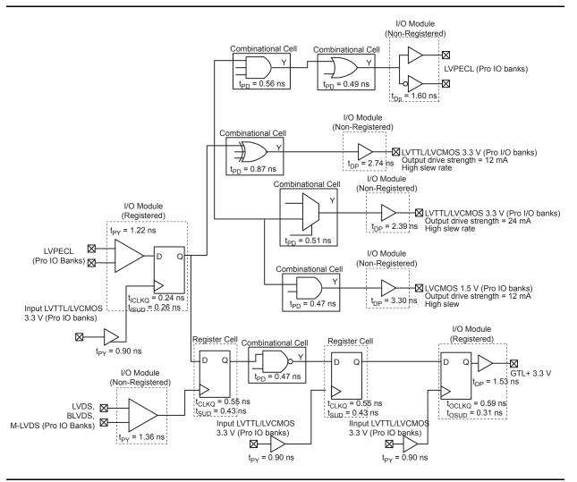
Figure 2-115 • Timing Model Operating Conditions: –2 Speed, Commercial Temperature Range (T<sub>J</sub> = 70°C), Worst-Case VCC = 1.425 V
