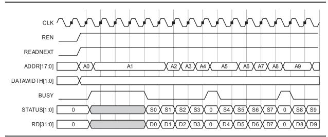
Figure 2-40 • Read Next Waveform (Non-Pipe Mode, 32-bit access)
