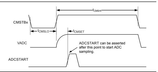
Figure 2-71 • Timing Diagram for Current Monitor Strobe
