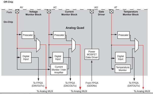
Figure 2-66 • Analog Quad Direct Connect
