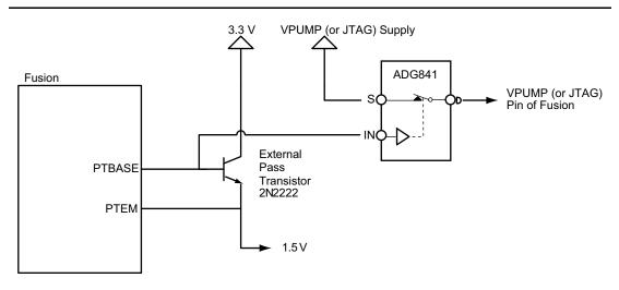
Figure 2-28 • Implementation to Control VPUMP
