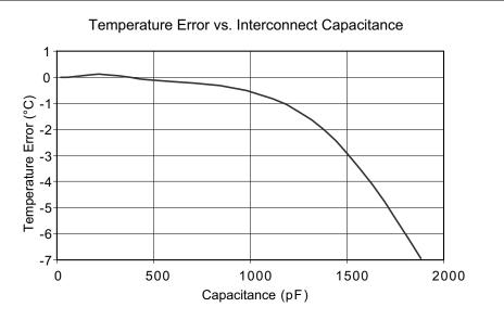
Figure 2-95 • Effect of External Sensor Capacitance
