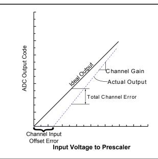
Figure 2-68 • Total Channel Error Example
