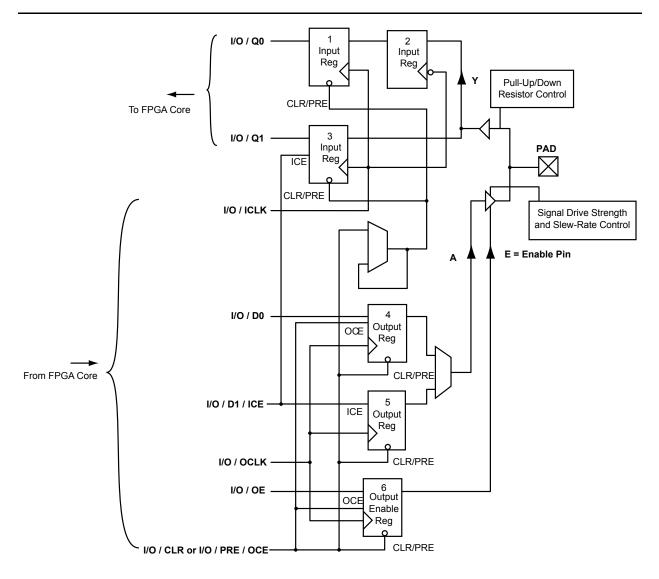
Note: Fusion I/Os have registers to support DDR functionality (see the "Double Data Rate (DDR) Support" section on page 2-139 for more information).
