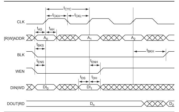
Figure 2-52 • RAM Write, Output Retained. Applicable to both RAM4K9 and RAM512x18.
