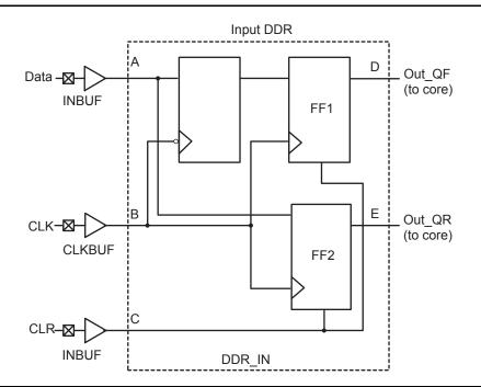
Figure 2-101 • DDR Input Register Support in Fusion Devices
