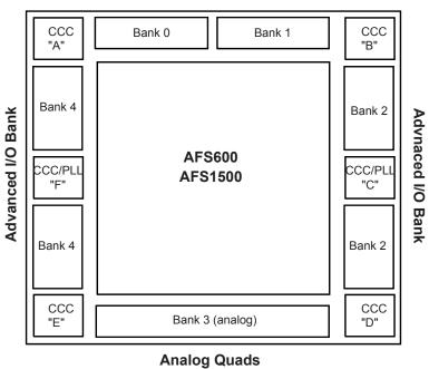
Figure 2-114 • Naming Conventions of Fusion Devices with Four I/O Banks
