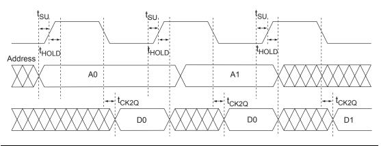
Figure 2-46 • FlashROM Timing Diagram
