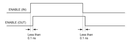
Figure 2-108 • Timing Diagram (option1: bypasses skew circuit)
