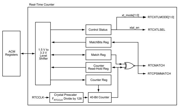
Figure 2-29 • RTC Block Diagram
