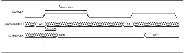
Figure 2-98 • ACM Read Waveform
