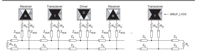
Figure 2-135 • BLVDS/M-LVDS Multipoint Application Using LVDS I/O Buffers
