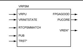
Note: \*Signals are hardwired internally and do not exist in the macro core.
