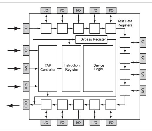
Figure 2-146 • Boundary Scan Chain in Fusion
