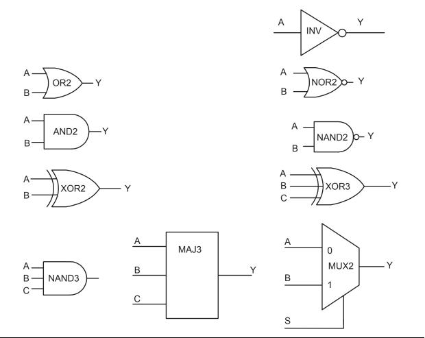
Figure 2-3 • Sample of Combinatorial Cells
