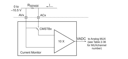
Figure 2-73 • Negative Current Monitor
