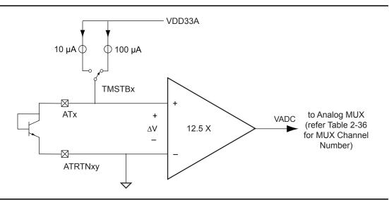
Figure 2-77 • Block Diagram for Temperature Monitor Circuit
