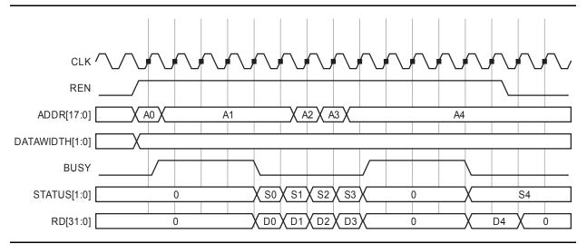
Figure 2-38 • Read Waveform (Non-Pipe Mode, 32-bit access)
