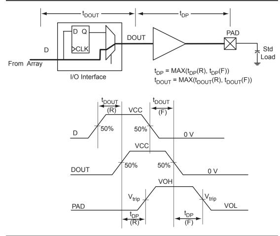
Figure 2-117 • Output Buffer Model and Delays (example)
