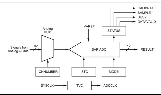
Figure 2-80 • ADC Simplified Block Diagram
