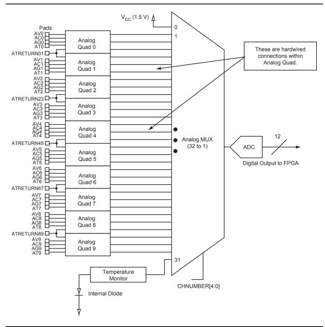
Figure 2-79 • ADC Block Diagram
