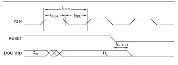
Figure 2-55 • RAM Reset. Applicable to both RAM4K9 and RAM512x18.
