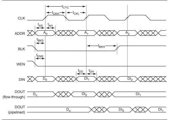
Figure 2-53 • RAM Write, Output as Write Data (WMODE = 1). Applicable to RAM4K9 Only.
