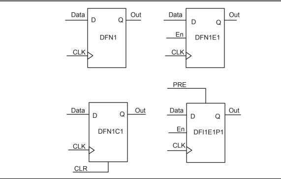
Figure 2-5 • Sample of Sequential Cells
