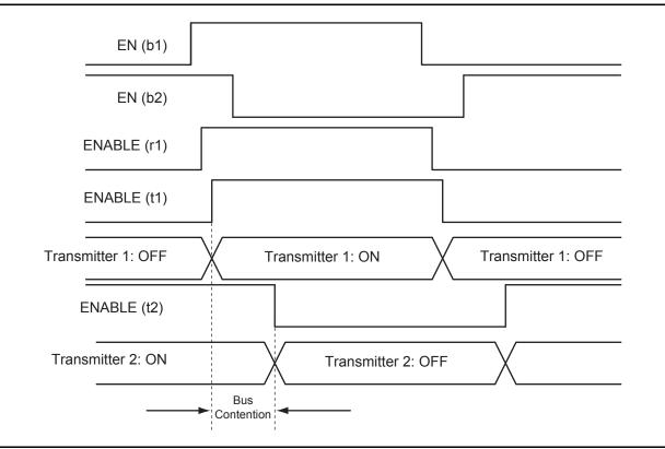
Figure 2-111 • Timing Diagram (bypasses skew circuit)
