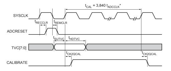
Note: \*Refer to EQ 15 on page 2-107 for the calculation on the period of ADCCLK, t<sub>ADCCLK</sub>.
