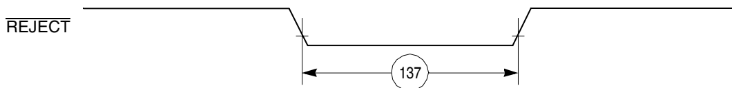
Figure 65. CAM Interface \overline{\text{REJECT}} Timing Diagram
