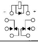
CONTACT RATING: LOW LEVEL TO 1A 28 VDC RESISTIVE 100,000 OPERATIONS
