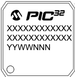
100-Lead TQFP (12x12x1 mm)
