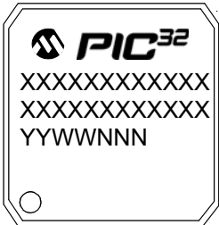
100-Lead TQFP (12x12x1 mm)
