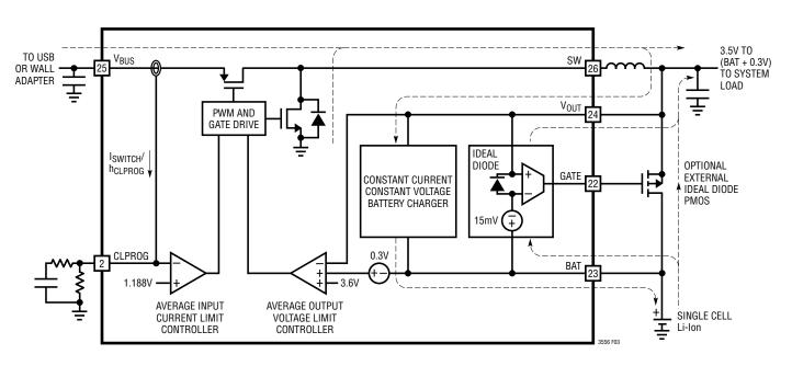
Figure 3. PowerPath Block Diagram
