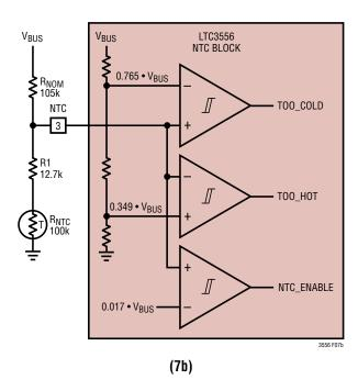
Figure 7. NTC Circuits
