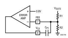
Figure 5. Error Amplifier with Type I Compensation
