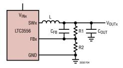
Figure 4. Buck Converter Application Circuit
