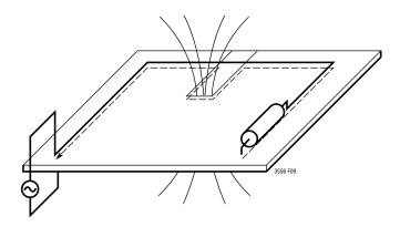
Figure 9. Higher Frequency Ground Currents Follow Their Incident Path.
