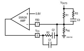
Figure 6. Error Amplifier with Type III Compensation
