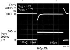
Start-Up Sequencing with SEQ = 0V  $V_{IN1} = V_{IN2} = V_{IN3} = 4.2V$  All Outputs Loaded with 5mA
