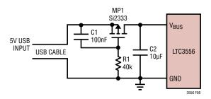
Figure 8. USB Soft Connect Circuit
