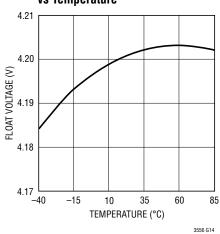
Low-Battery (Instant On) Output Voltage vs Temperature
