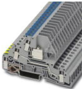
Installation ground terminal block, Screw connection, cross section: 0.2 mm<sup>2</sup> - 4 mm<sup>2</sup>, AWG: 24 - 12, width: 6.2 mm, color: gray, mounting type: NS 35/7,5, NS 35/15
