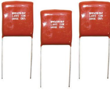
**Type DPM** radial-lead, metallized polypropylene capacitors boast non-inductive windings with welded lead terminations which handle high continuous currents. The low ESR and low ESL are a glove fit for high frequency and switching power supply applications.
