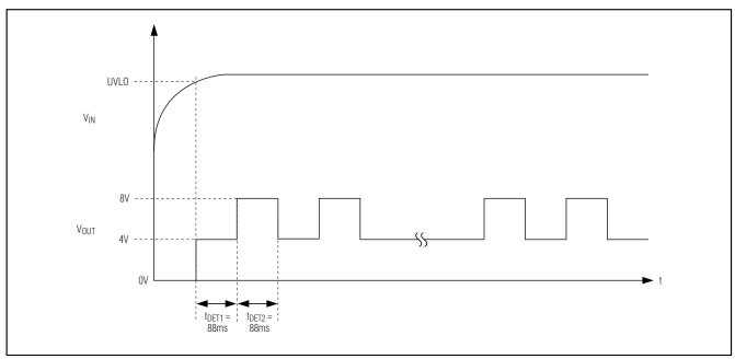
Figure 5. PD Detection with an Invalid PD Signature
