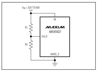
Figure 7. Setting Undervoltage Lockout with an External Resistive-Divider
