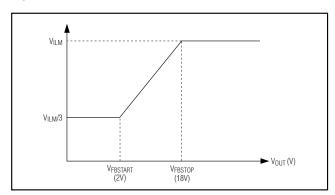
Figure 8. Current Foldback Characteristic
