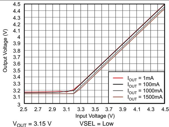
Figure 37. TPS61281A DC Output Voltage vs Input Voltage
