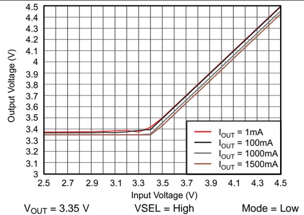
Figure 38. TPS61281A DC Output Voltage vs Input Voltage
