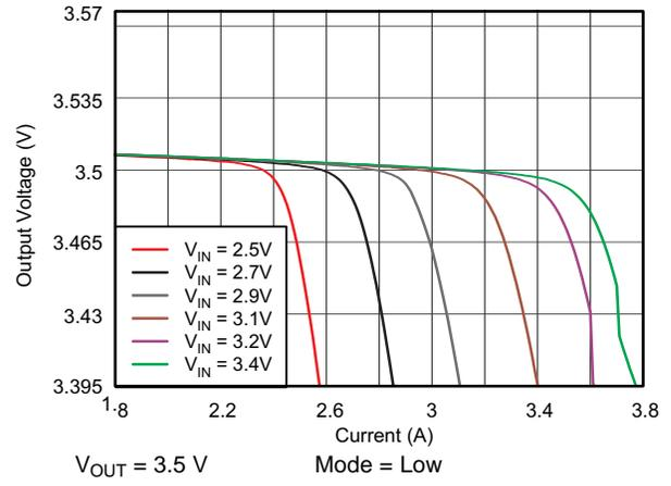
Figure 56. TPS61282A DC Output Voltage vs Output Current
