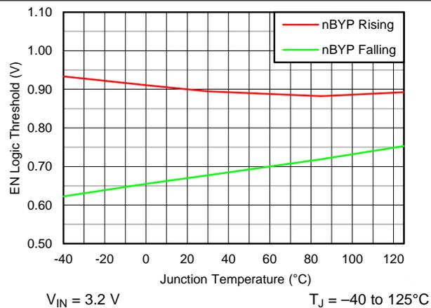
Figure 14.  $\overline{BYP}$  Logic High Threshold Rising/Falling vs Junction Temperature
