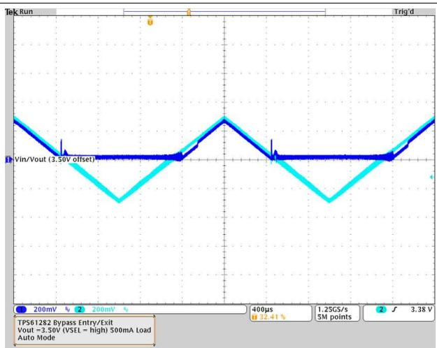
Figure 59. Boost to Pass-Through Mode Exit / Entry
