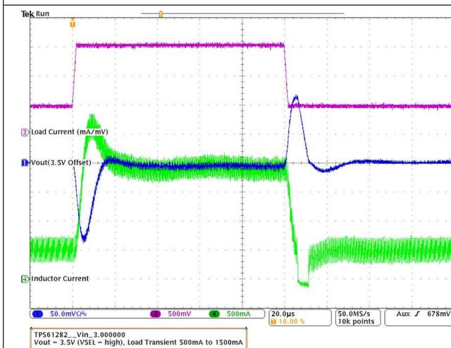
Figure 63. TPS61282A Load Transient Response In PWM Operation
