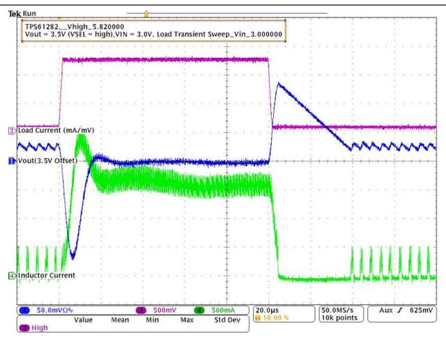
Figure 64. TPS61282A Load Transient Response In PFM/PWM Operation
