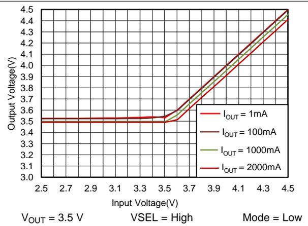
Figure 58. TPS61282A DC Output Voltage vs Input Voltage
