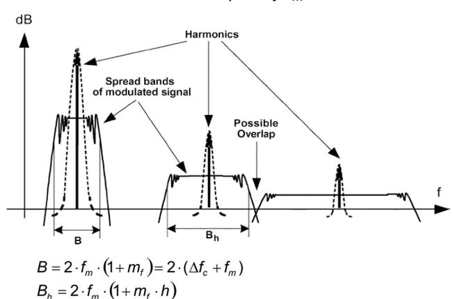
**Figure 16. Spread Bands of Harmonics in Modulated Square Signals <sup>(1)</sup>**
