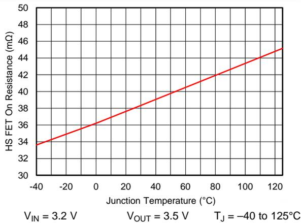
Figure 3. High side  $R_{ds(on)}$  vs Junction Temperature
