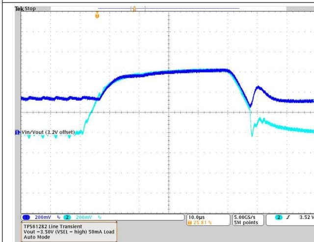
Figure 43. TPS61282A Forced Pass-Through to Boost Mode Transition
