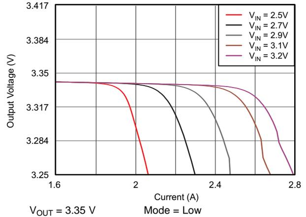
Figure 36. TPS61281A DC Output Voltage vs Output Current
