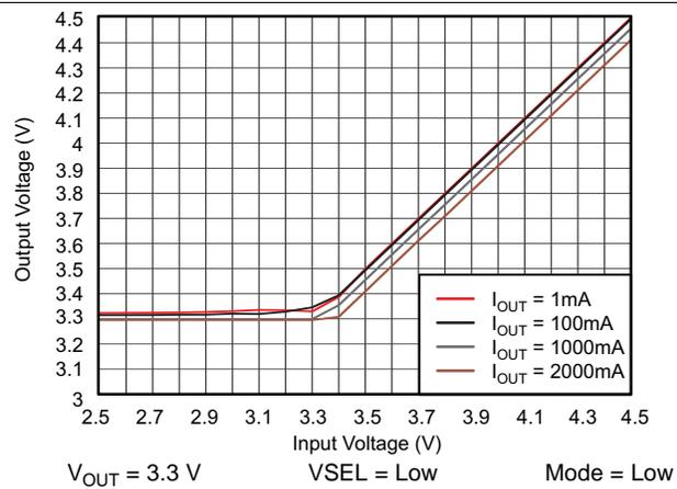
Figure 57. TPS61282A DC Output Voltage vs Input Voltage
