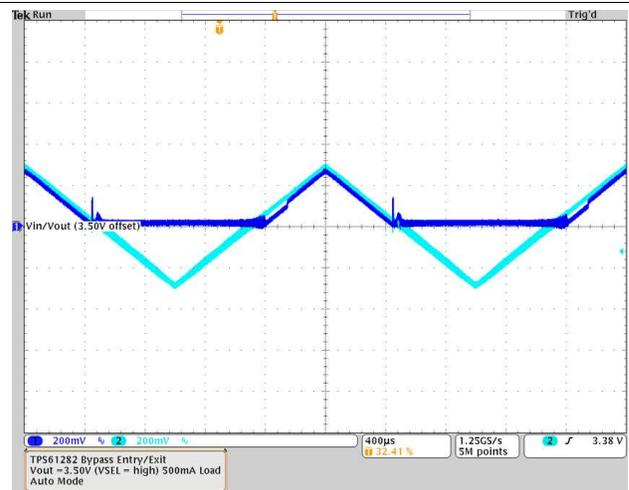
Figure 40. Boost to Pass-Through Mode Exit / Entry
