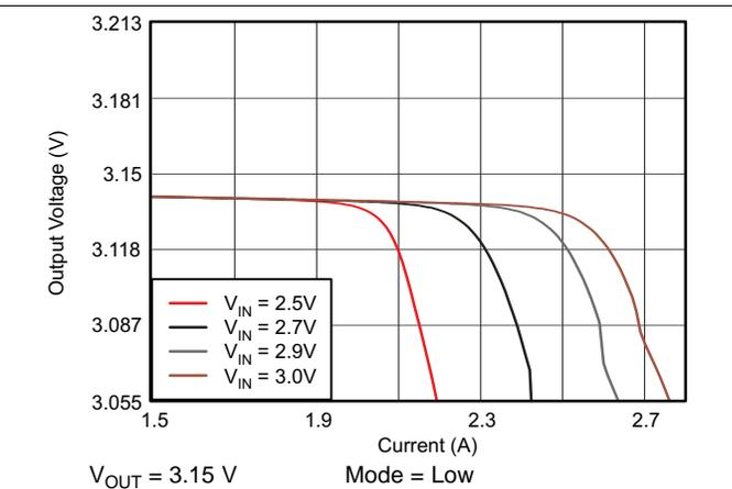
Figure 34. TPS61281A DC Output Voltage vs Output Current
