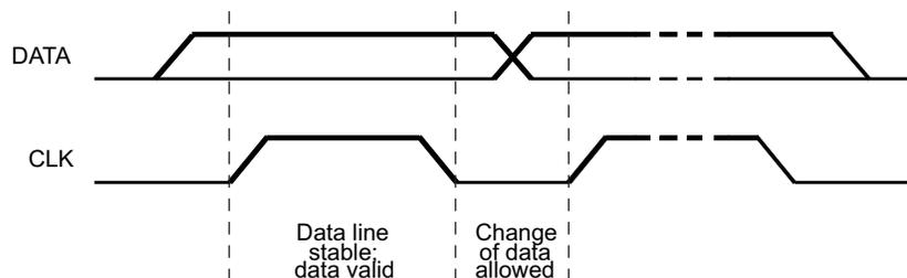
Figure 21. Bit Transfer on the Serial Interface
