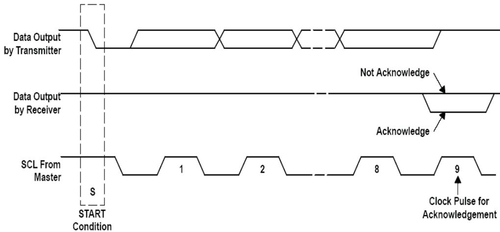
Figure 22. Acknowledge on the I<sup>2</sup>C Bus
