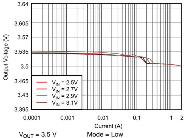
Figure 55. TPS61282A DC Output Voltage vs Output Current
