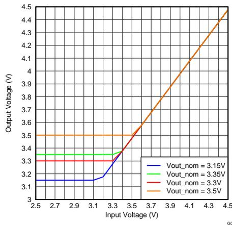
**Figure 18. DC Output Voltage vs. Input Voltage**
