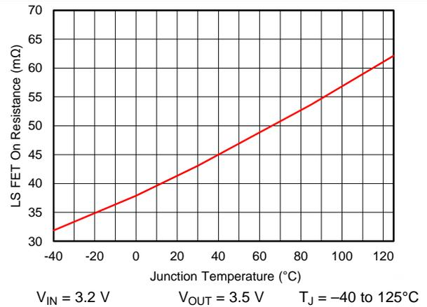
Figure 4. Low side  $R_{ds(on)}$  vs Junction Temperature
