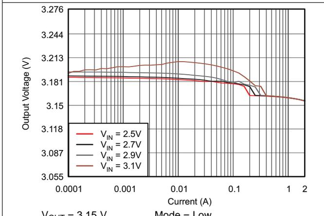
Figure 33. TPS61281A DC Output Voltage vs Output Current
