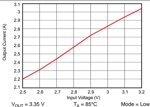
Figure 39. TPS61281A Maximum Output Current vs Input Voltage
