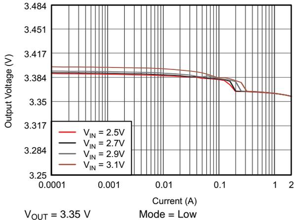
Figure 35. TPS61281A DC Output Voltage vs Output Current
