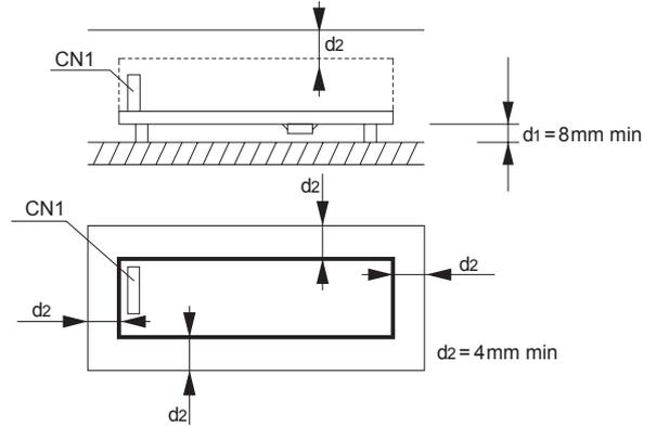
■ (F) mounting should be operated by Forced air.
