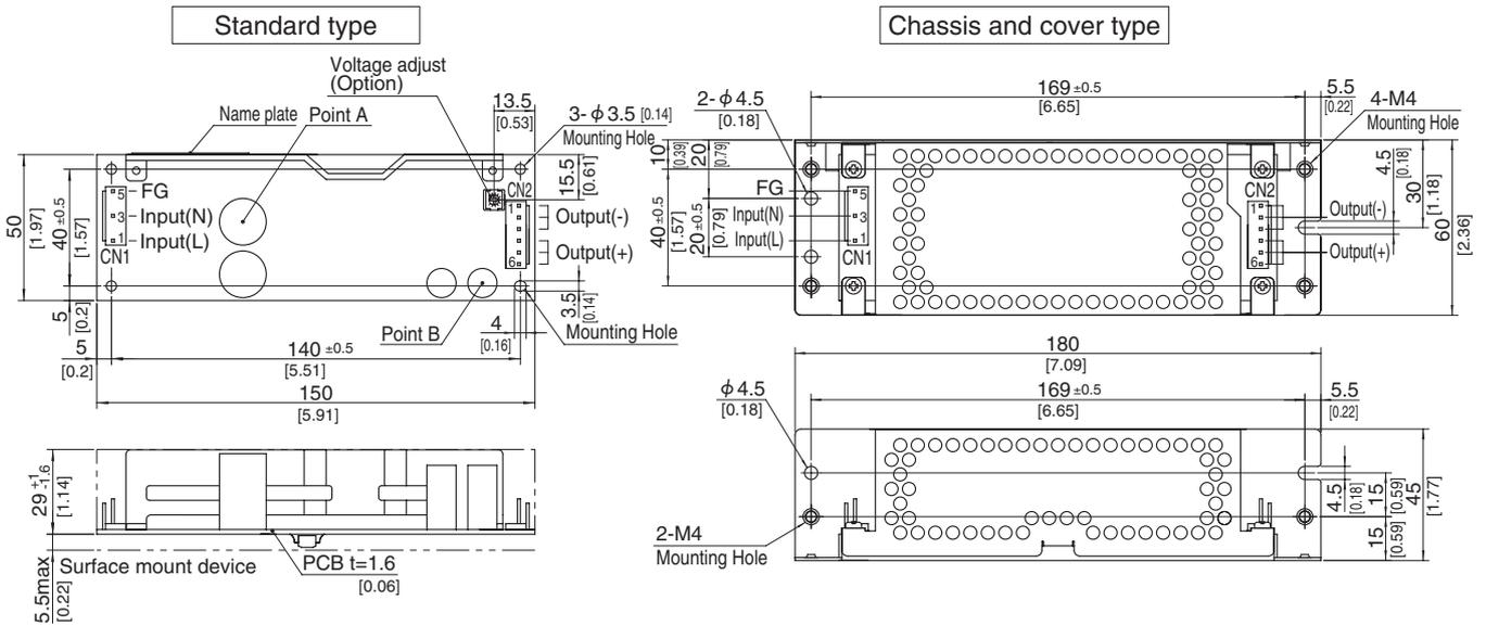
※ This power supply is manufactured by SMD technology. The stress to P.C.B like twisting or bending causes the defect of the unit, so handle the unit with care. Take care for SMD parts on the back to come in contact because of the vibration and not to break down.
