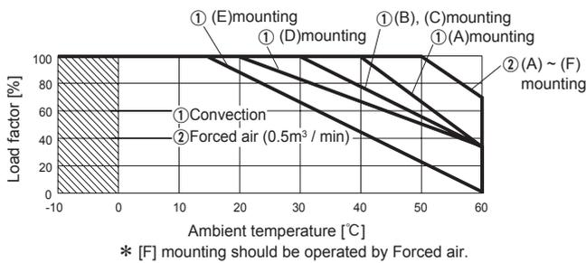
● LGA240A-□-SN (with Chassis & Cover) Ambient temperature derating curve
