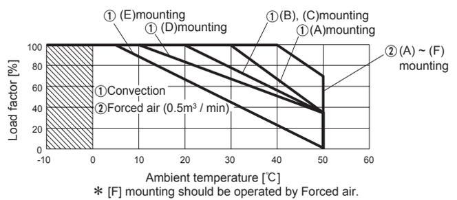
■ The operative ambient temperature is different by with / without chassis cover or mounting position.
