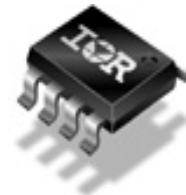
8-Lead SOIC AUIRS2301S
