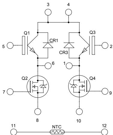
Top switches : Trench + Field Stop IGBT®
