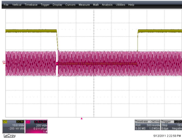
CH1:Vo (10 V/div) CH2:Vin (200 V/div) Figure 11: AC drop out 50 mS@115 VAC (50 mS/div), Vo restart
