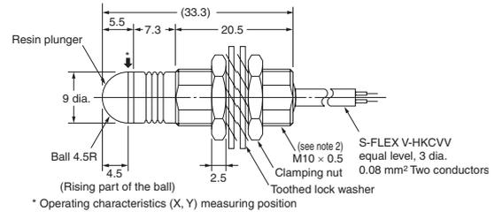
\* Operating characteristics (X, Y) measuring position
