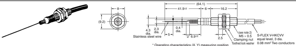
Note: 1. Unless otherwise specified, a tolerance of ±0.4 mm applies to all dimensions.
