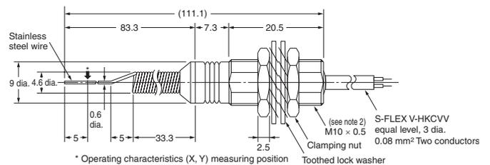
\* Operating characteristics (X, Y) measuring position
