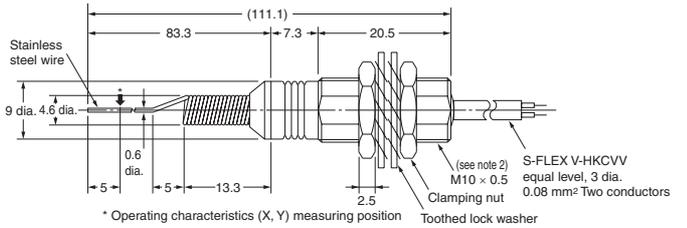
\* Operating characteristics (X, Y) measuring position
