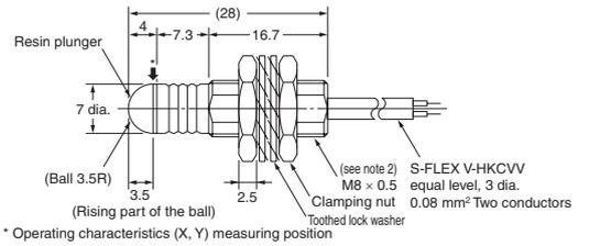
\* Operating characteristics (X, Y) measuring position
