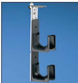
Final assembly is a second-level installation consisting of one threaded rod bracket, one chaining bracket, and two J-hooks for clarity.
