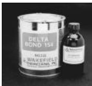
**DeltaBond™ 154** is a medium viscosity, aluminum-filled resin with the best thermal conductivity of this series. It is, however, neither a good electrical insulator nor conductor. Its principal application is that of a good thermal mechanical adhesive for applications such as bonding fins to base plates or structural mounting blocks or brackets to heat sinks. Shelf life: 2 years.
