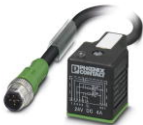
Sensor/actuator cable, 5-position, PUR/PVC, black RAL 9005, Plug straight M12, A-coded, on Valve connector AD (pressure switch), with 2 LEDs, cable length: 1.5 m
