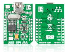
USB SPI click<sup>TM</sup> is an accessory board in **mikroBUS**<sup>TM</sup> form factor. It's a compact and easy solution for adding SPI serial communication via USB cable. It features **MCP2210** USB-to-SPI protocol converter with GPIO as well as USB MINI B connector. USB SPI click<sup>TM</sup> communicates with target board via SPI interface as a master device. The board is designed to use 3.3V or 5V power supply. It has a LED diode (GREEN) that indicates the presence of power supply.
