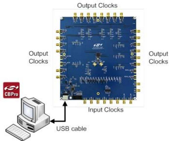
**Figure 6. EVB Connection Diagram**
