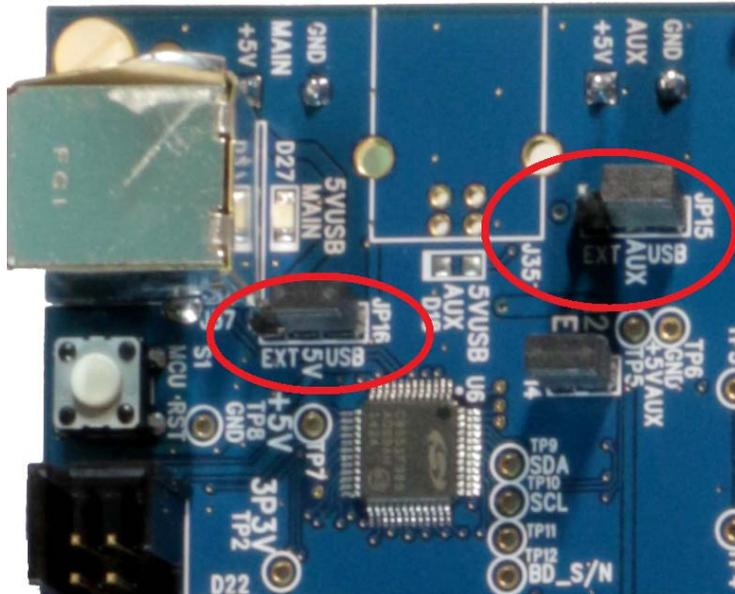
**Figure 7. JP15-JP16 Standard Jumper Shunt Installation**
