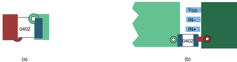
Figure 21. Typical Decoupling Capacitor Layouts
