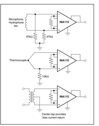
FIGURE 5. Providing an Input Common-Mode Current Path.
