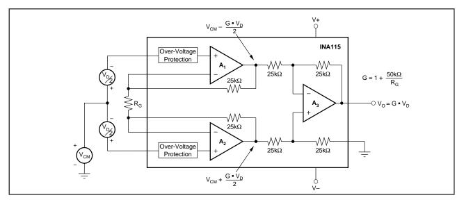
FIGURE 6. Voltage Swing of A<sub>1</sub> and A<sub>2</sub>.
