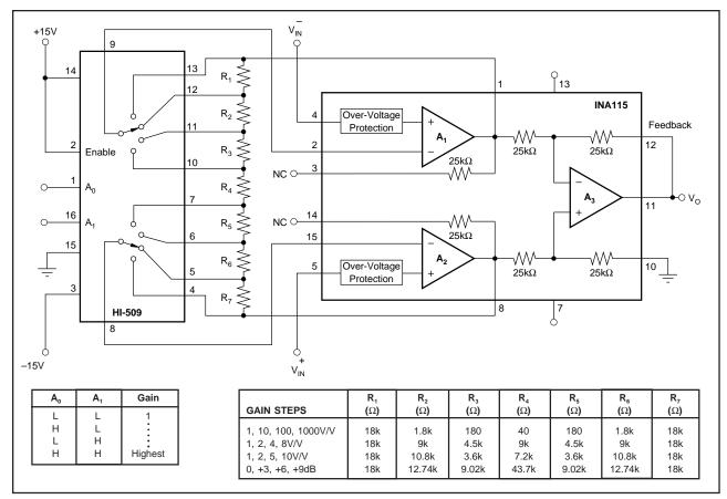
FIGURE 3. Switched-Gain Instrumentation Amplifier (improved gain drift).
