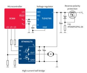
Applications: high current DC- or brushless DC (BLDC) motor drives for use in applications like:
