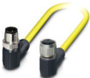
Sensor/actuator cable, 5-position, PVC, yellow, shielded, Plug angled M12 SPEEDCON, coding: A, on Socket angled M12 SPEEDCON, coding: A, cable length: 0.5 m
