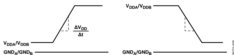
Figure 14. Transient Immunity Waveforms—Output Supplies
