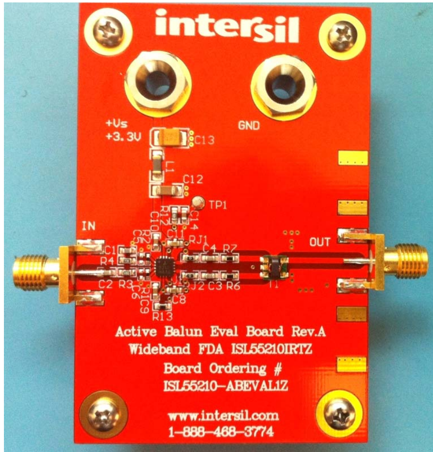
FIGURE 5. POPULATED BOARD AS DELIVERED FROM INTERSIL
