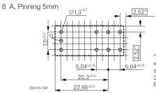
\*) With the recommended PCB hole sizes a grid pattern from 2.5mm to 2.54mm can be used.
