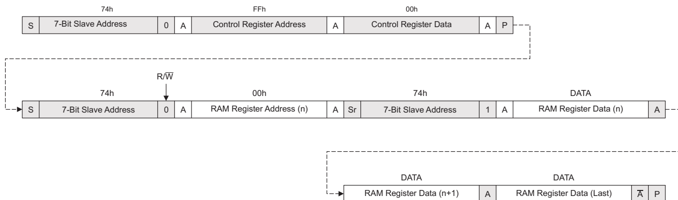
Figure 5-34. Reading from Multiple RAM Registers
