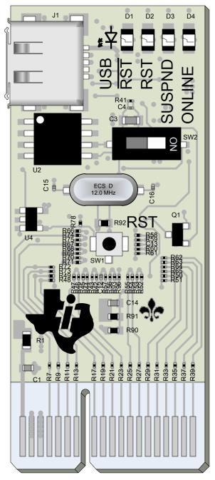
Figure 2. USB Dongle Board
