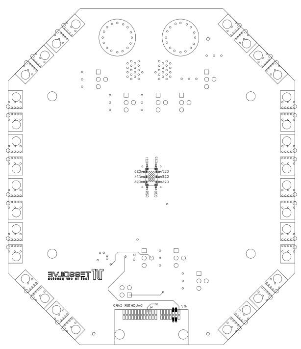
Figure 12. SN65LVCP1414 Board Layout: Bottom Signal (Layer 4)
