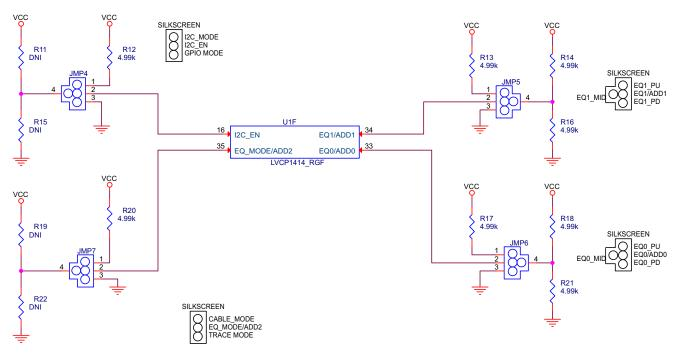
Figure 6. SN65LVCP1414 EVM Schematic, Sheet 3 I<sup>2</sup>C Controls
