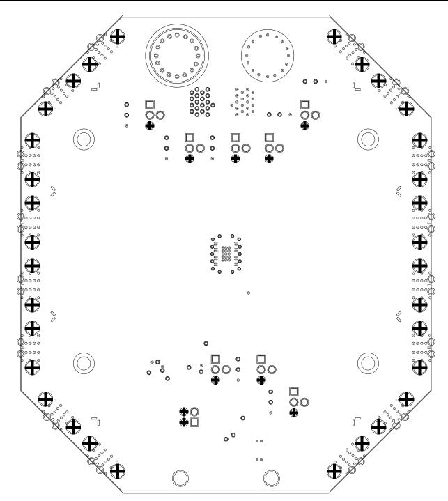
Figure 10. SN65LVCP1414 Board Layout: Internal Ground (Layer 2)
