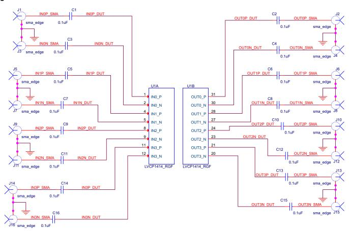
Figure 4. SN65LVCP1414 EVM Schematic, Sheet 1 Inputs and Outputs
