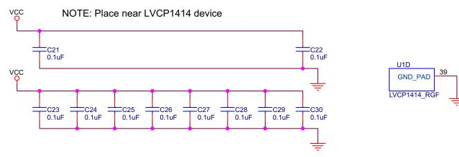
Figure 8. SN65LVCP1414 EVM Schematic, Sheet 5 Power
