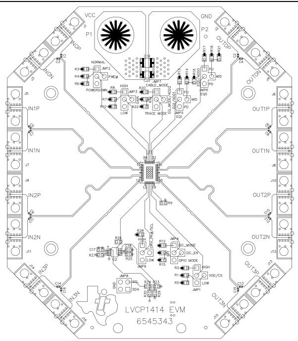
Figure 9. SN65LVCP1414 Board Layout: Top Signal (Layer 1)
