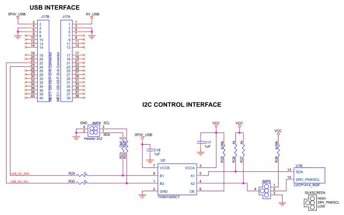
Figure 7. SN65LVCP1414 EVM Schematic, Sheet 4 I<sup>2</sup>C Communications
