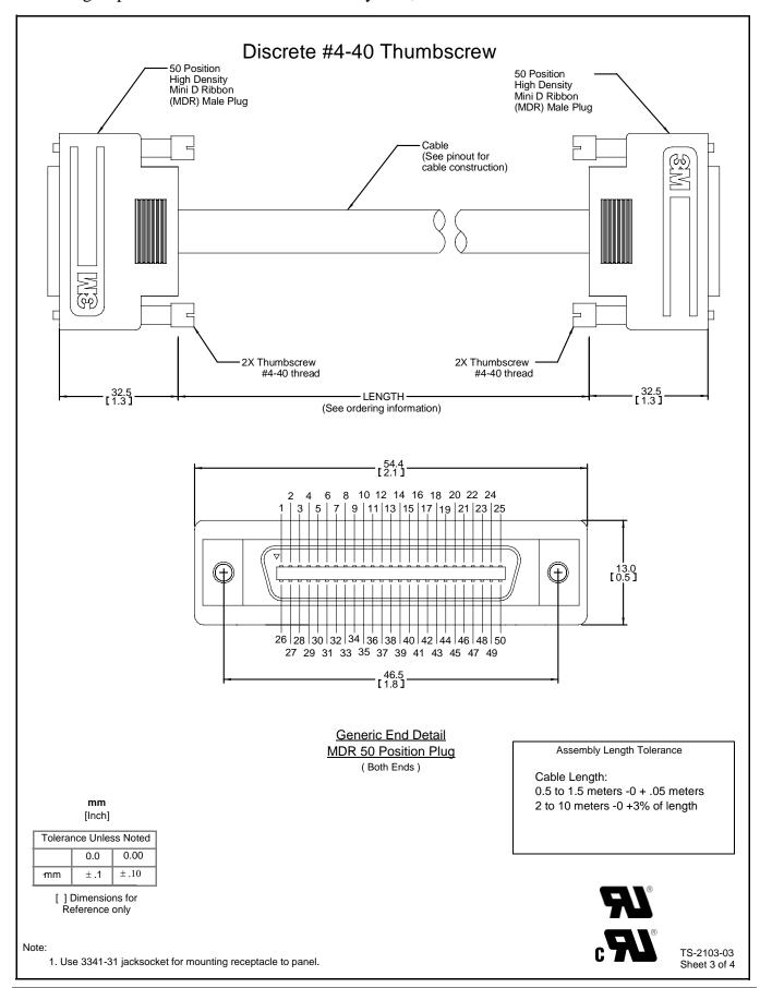
.050" High Speed Video Data Transmission System, 50 Position 14X50-SZWB-XXX-0NC
