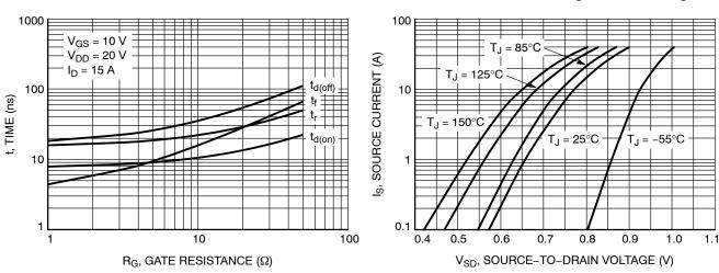
Figure 11. Resistive Switching Time Variation vs. Gate Resistance
