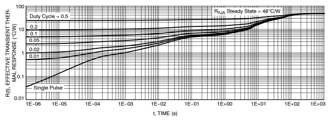
Figure 14. Thermal Impedance (Junction-to-Ambient)
