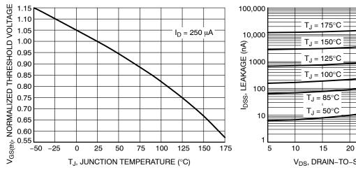
Figure 7. Threshold Voltage Variation with Temperature
