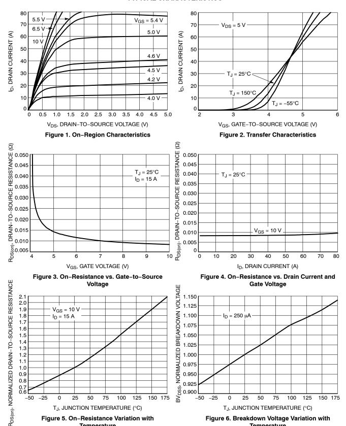
Figure 6. Breakdown Voltage Variation with
