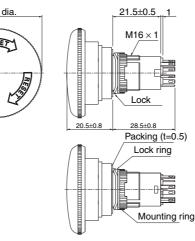
When applying a coating such as paint to the panel, dimensions after the coating must satisfy the specified dimensions.
