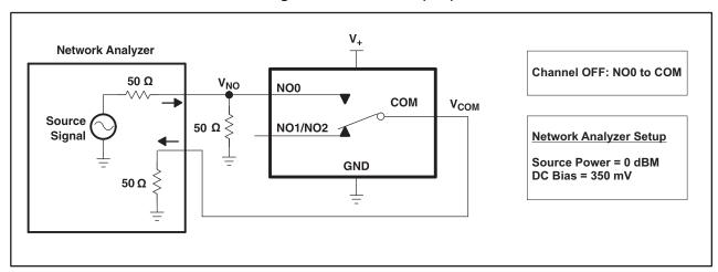
Figure 19. OFF Isolation (O<sub>ISO</sub>)
