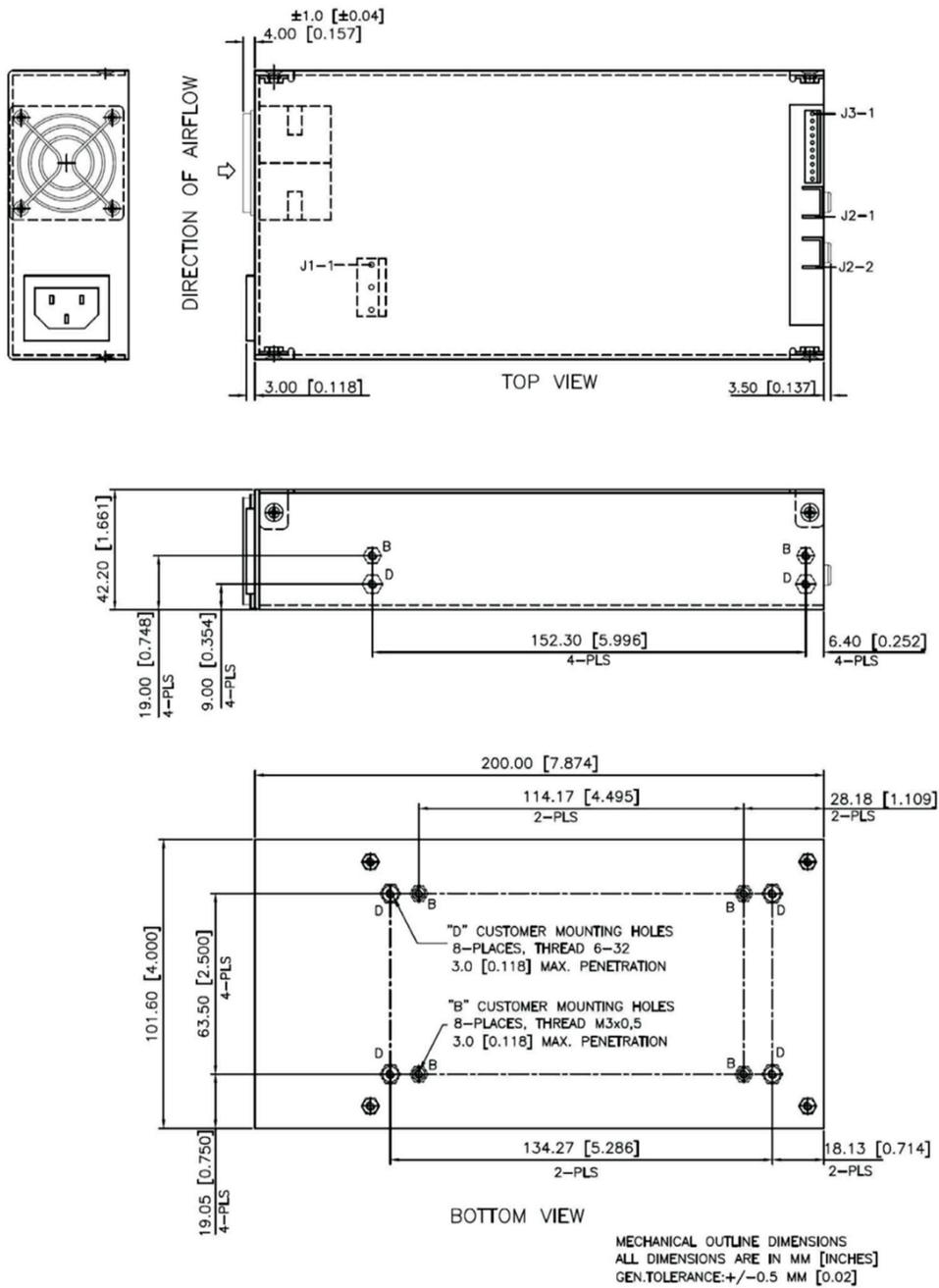
Figure 4 - Mechanical Drawing (With Side Fan Mounting)
