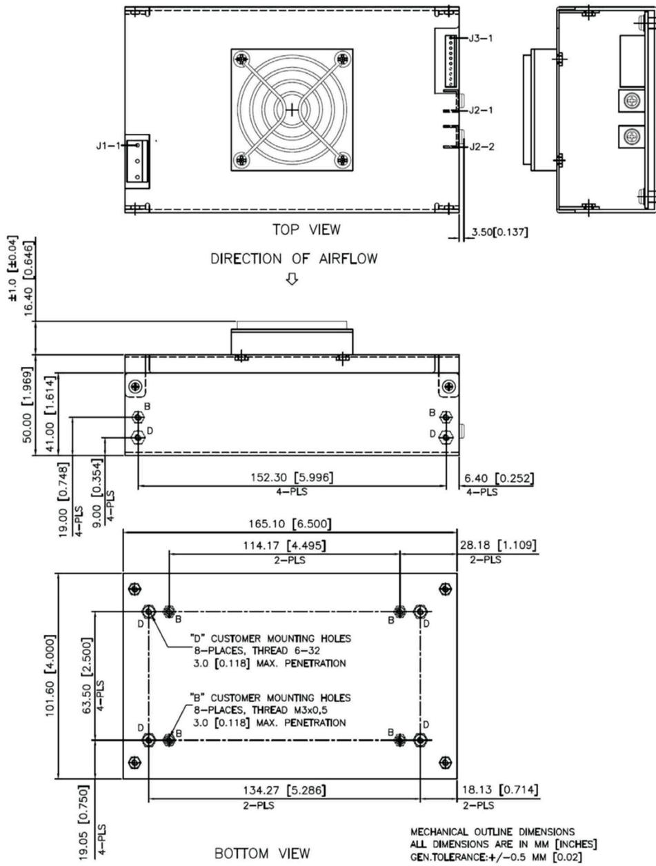
Figure 3 - Mechanical Drawing (With Top Fan Mounting)
