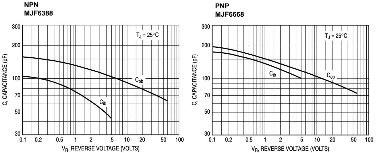
Figure 8. Typical Capacitance
