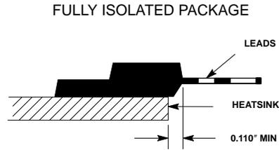
Figure 14. Mounting Position
