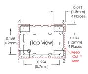
\* Do not route any traces in the keep out area. It is recommended the next layer under the keep out area is to be ground plane.
