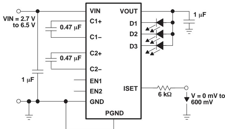
**Figure 13. Analog Dimming Connections Using ISET Pin**
