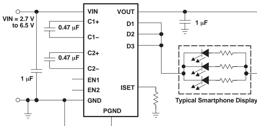
Figure 12. Typical Application With Resistors in Parallel
