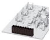
Header, Nominal current: 12 A, Rated voltage (III/2): 320 V, Number of positions: 5, Pitch: 5 mm, Color: black, Contact surface: Tin, Mounting: THR soldering, User information and design recommendations for through hole reflow technology can be found under "Downloads"
