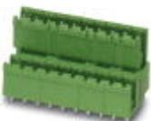
Header, Nominal current: 10 A, Rated voltage (III/2): 320 V, Number of positions: 5, Pitch: 5 mm, Color: green, Contact surface: Tin, Mounting: Wave soldering, Can be aligned! Mounting flange: Order No. 1836477, 1836480. In combination with MVSTB or FKCV plug components, both an MVSTBW (or FKCVW) and an MVSTBR plug (or FKCVR) must be used. Combination with TMSTBP plug components is not possible!
