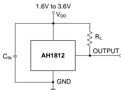
Note: 4. C<sub>IN</sub> is for power stabilization and to strengthen the noise immunity, the recommended capacitance is 10nF to 100nF. R<sub>L</sub> is the pull-up resistor, the recommended resistance is 10k $\Omega$  to 100k $\Omega$ .
