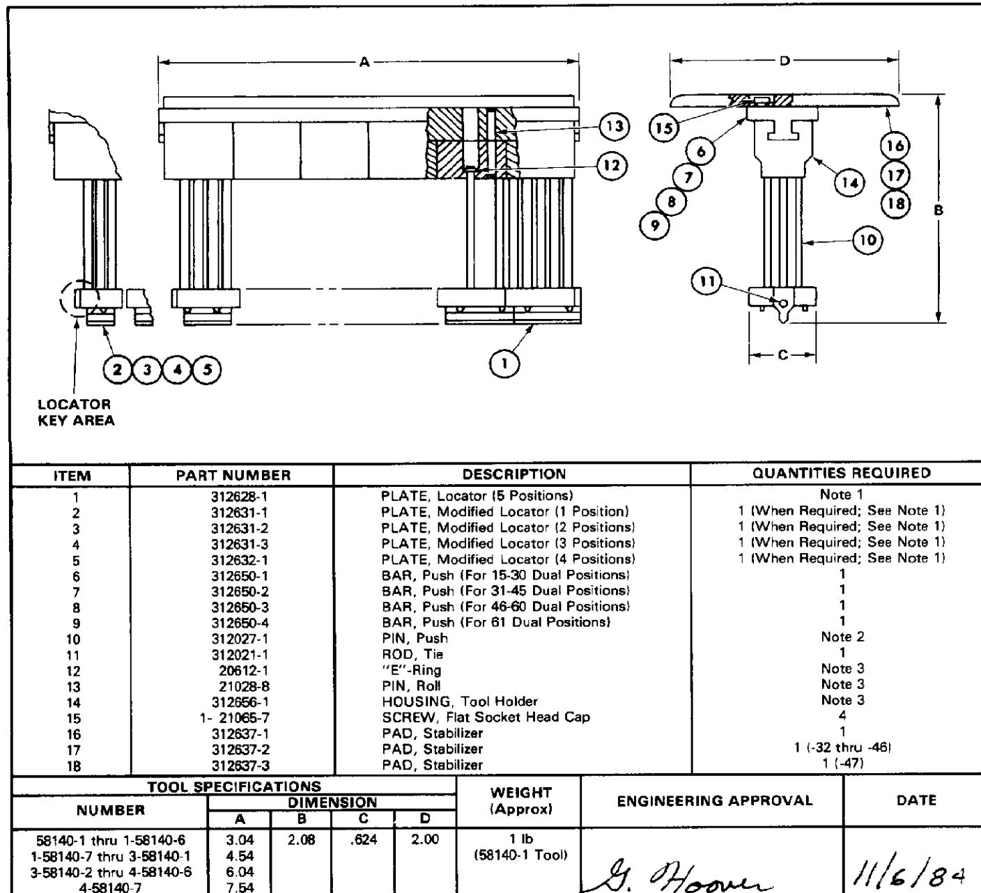
NOTE 1: THE NUMBER OF LOCATOR PLATES REQUIRED FOR A GIVEN TOOL IS DETERMINED BY DIVIDING THE NUMBER OF DUAL CONTACT POSITIONS BY FIVE. THE REMAINDER OF POSITIONS, IF ANY, WILL REQUIRE AN APPROPRIATE MODIFIED LOCATOR PLATE.
