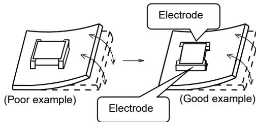
(2) Components location on PCB separation
