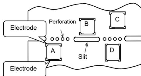
(3) Mounting components near screw holes
