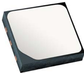
Figure 7. Si7023 with Factory-Installed Protective Cover
