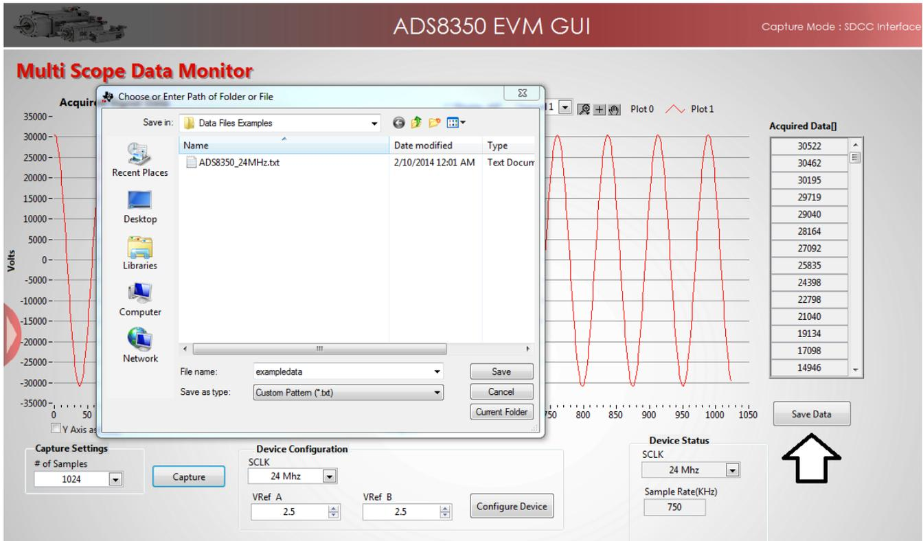
Figure 22. Saving Data to a Text File
