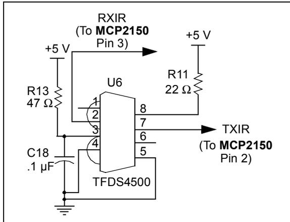
The optical transceiver logic can be implemented with discrete components for cost savings. Care must be taken in the design and layout of the photo detect circuit, due to the small signals that are being detected and their sensitivity to noise. A discrete implementation of the optical transceiver logic is implemented on the MCP2120 and MCP2150 Developer's Kit boards.
