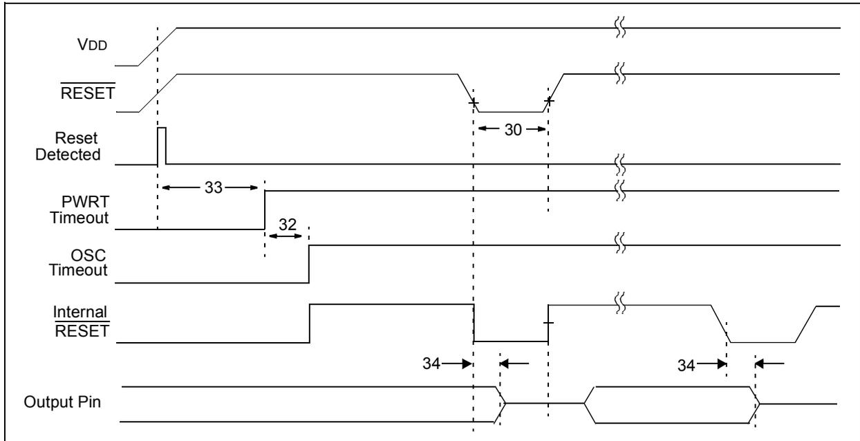
**TABLE 4-5:  $\overline{\text{RESET}}$  AND DEVICE RESET REQUIREMENTS**
