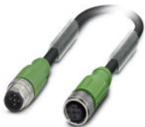
Sensor/actuator cable, 5-position, PUR halogen-free, black-gray RAL 7021, shielded, Plug straight M12, A-coded, on Socket straight M12, A-coded, cable length: 1.5 m
