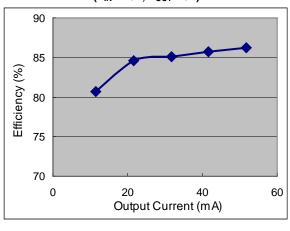
Efficiency vs. Output Current (V<sub>IN</sub> = 15V, V<sub>OUT</sub> = 3.3V)
