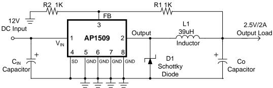
$$V_{OUT} = V_{FB} \times (1 + \frac{R1}{R2})$$
