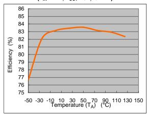
AP1509 Efficiency vs. Temperature  $(V_{IN} = 12V, V_{OUT} = 3.3V, Io = 2A)$
