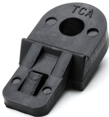
Lashing Tie Mount, .73" x 1.5", .25" Screw, PA66HS, Black, 100/pkg
